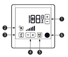
1 Temperature setpoint: Set the desired temperature
